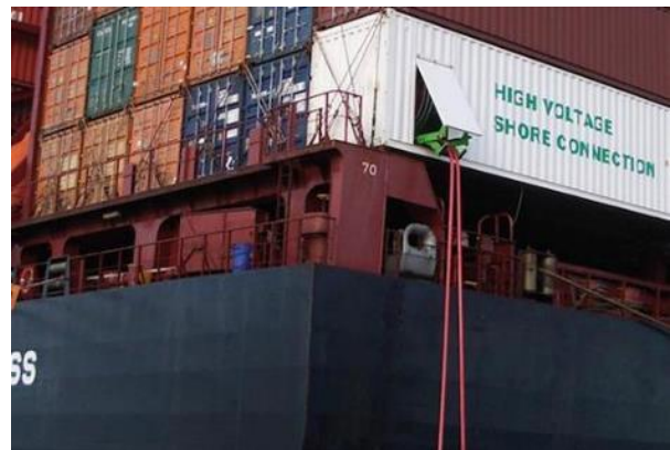
Figure 3.118 and Figure 3.119– Other example of onboard OPS fixed CMS - containership HVSC cable reel onboard.
