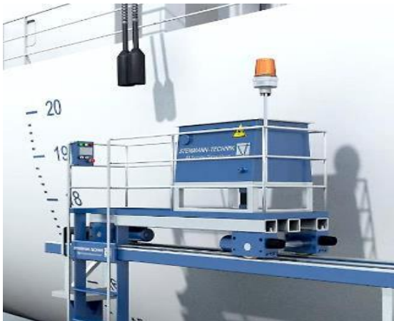
Figure 3.121 and Figure 3.122– To provide for longitudinal flexibility at berth, a mobile socket-outlet junction box can be considered in order to allow for cables to be provided by the ship-side at the most convenient location.
