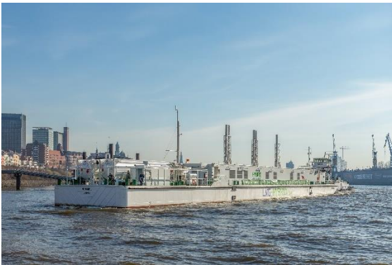
Figure 3.2 – Floating port generator.
