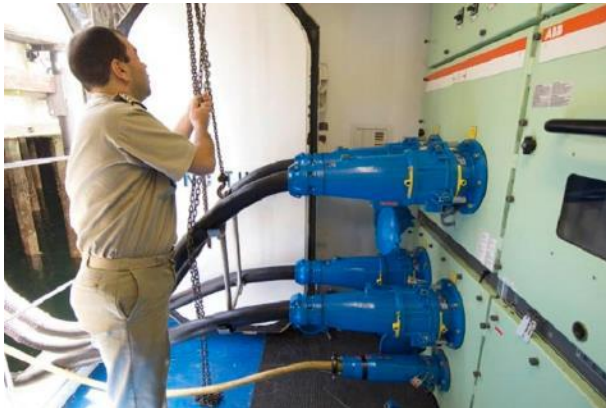
Figure 3.130– Ship side HVSC connector-inlet arrangement onboard a cruise ship including 4 parallel power cables + one neutral.
