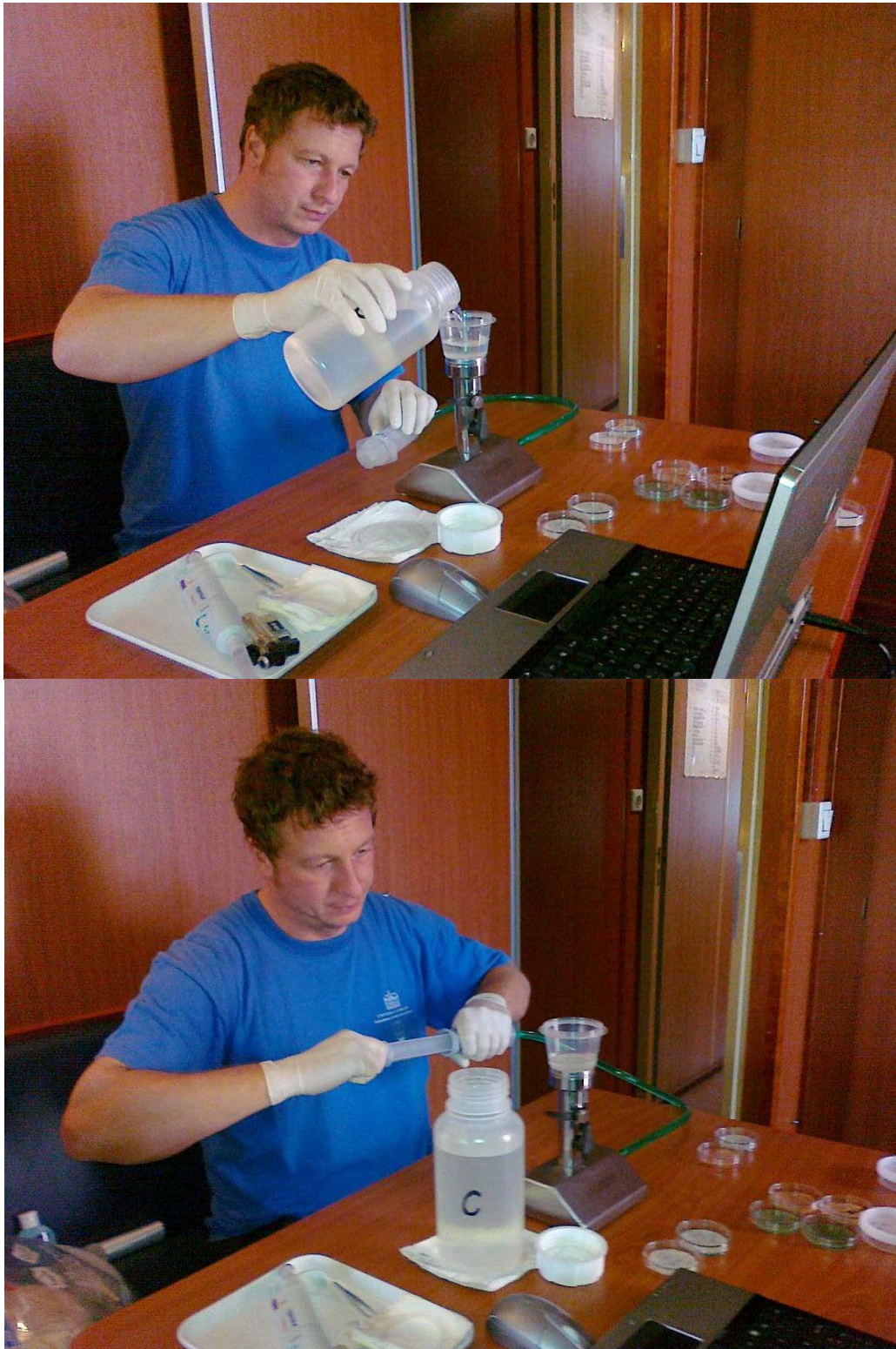
Figure 21 Onboard filtration of water for bacteria analysis using a Millipore stand.
