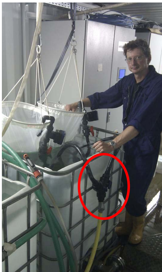
Figure 11 The flow splitter arrangement (red circle).
