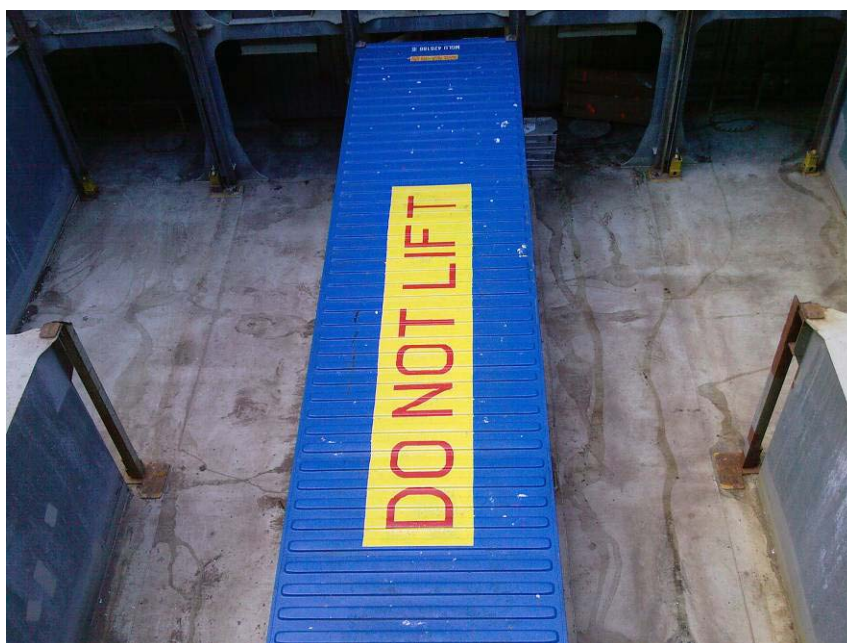
Figure 7 OPS installed in a container which is placed at the bottom of a cargo bay on the vessel.
