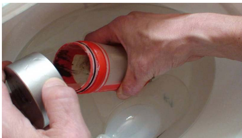
Figure 14 Metal lid screwed on cod-end for storage in 10 l bucket.
