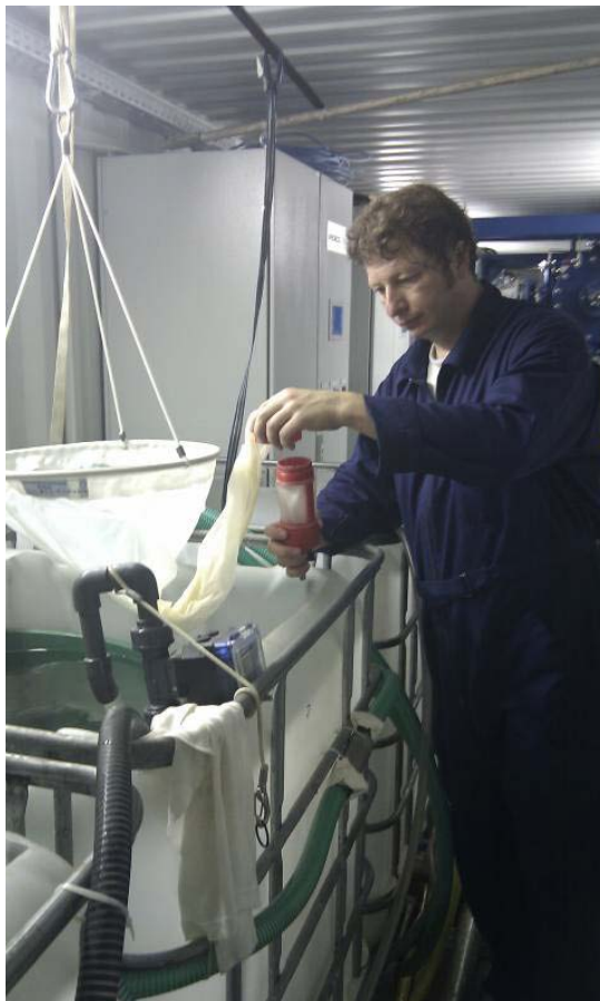
Figure 13 Cod-end with concentrated sample being unscrewed from plankton net.
