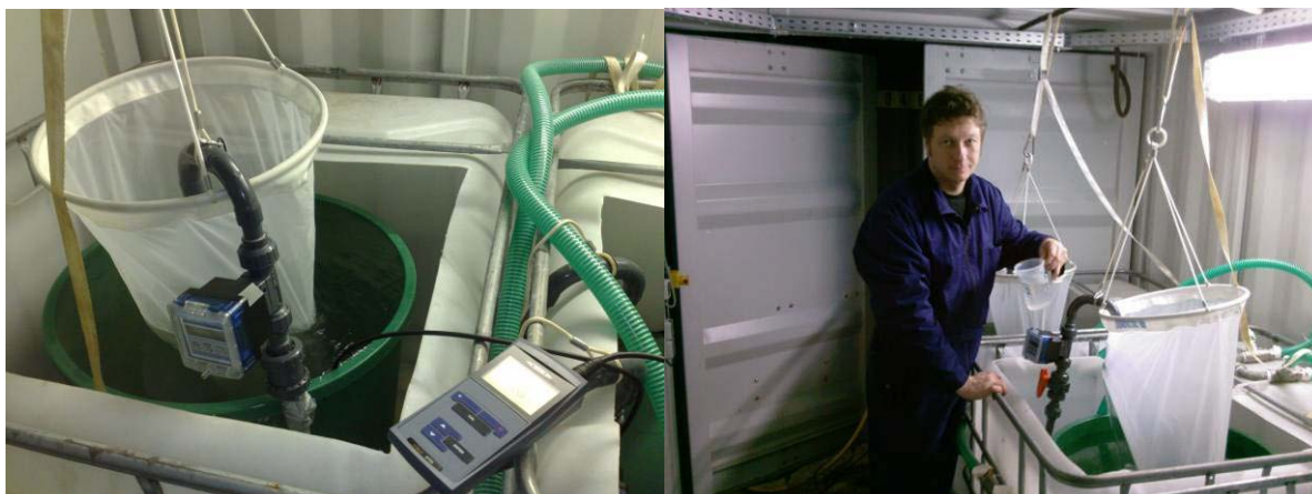
Figure 12 Plankton nets and flow meters used during the tests.
