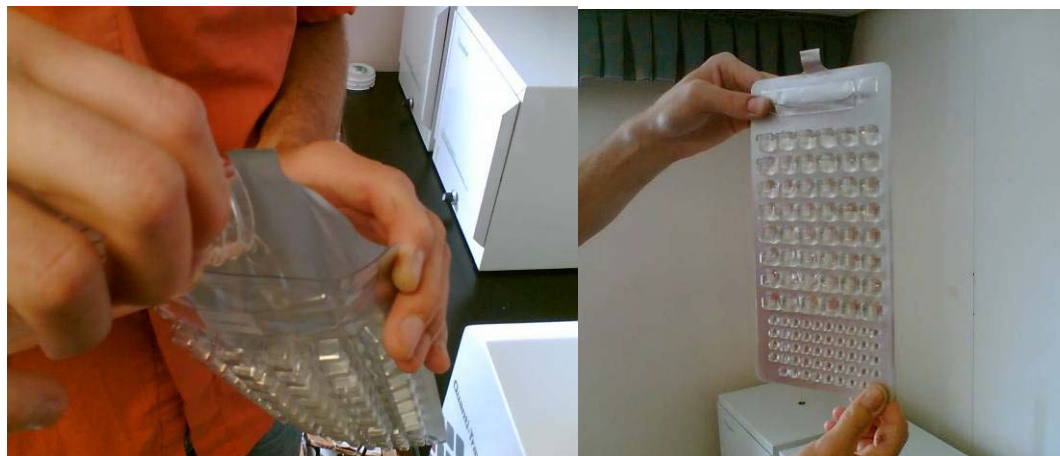
Figure 57 Sample transfer into IDEXX incubation plates (Quanti-Tray test plates).
