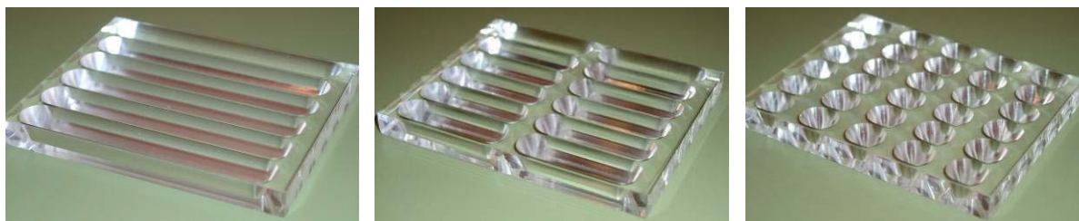
Figure 19 Newly designed counting chambers for organisms greater than or equal to 50 micrometres in minimum dimension. Photos courtesy of www.hydrobios.de .
