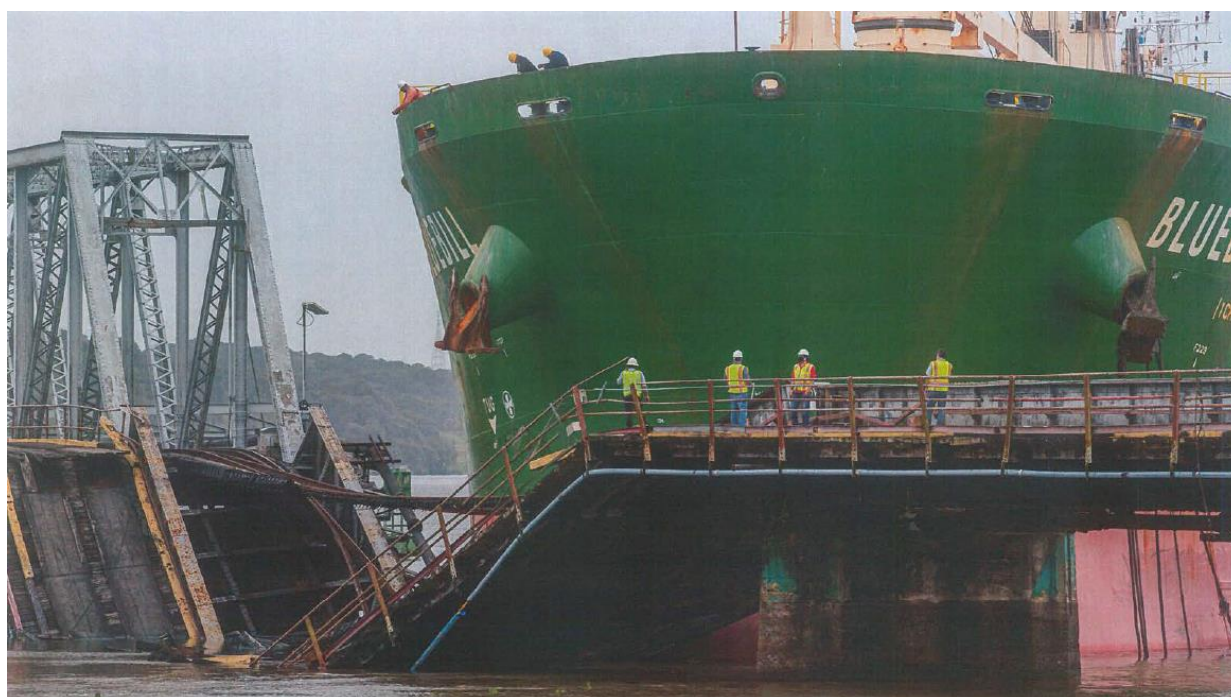
Contact of MV Bluebill with the Old Gaboa Railway Bridge in Panama Canal on 23/06/2020, following a loss of control / direction power.
