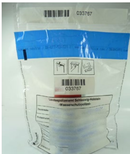
Figure 15: Different possibilities to seal samples (credits: upper left: SASEMAR Spain, lower left and right: BSH, Germany)
