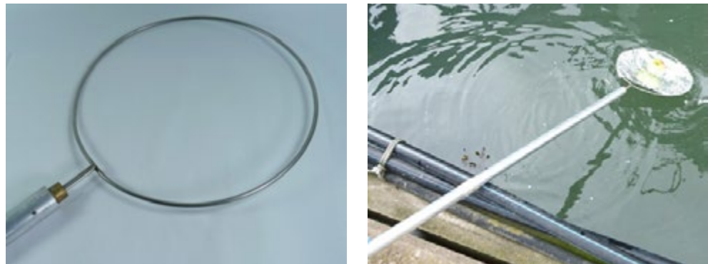
Figure 4: Custom-made sampling device to be used instead of a PE cornet (please note that during a sampling exercise, an apple was used as “tar ball” in the right-hand picture). Credits: U. Kraus, BSH
