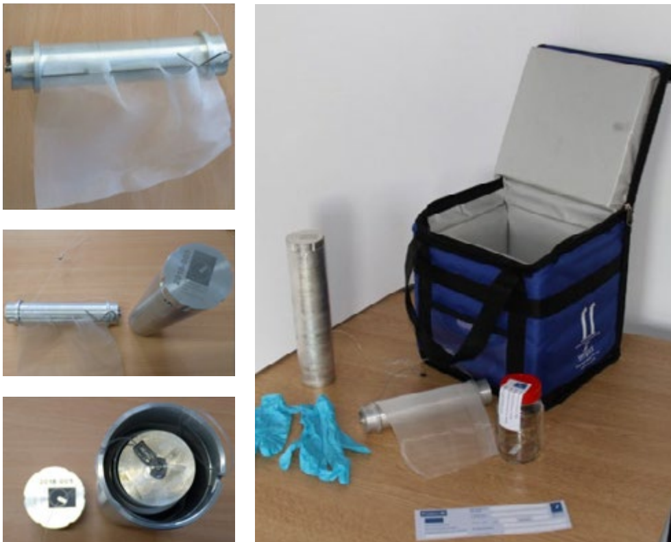
Figure 11: Example of a sampling device for oil sampling from heights with a floating body of aluminum. Upper left side: pre-assembled sampling device with mounted ETFE net. Left side middle and below: Pre-mounted sampling device in/beside the transportation cylinder. Credits: Pictures left side: BSH; picture right side: German Federal Police Department for Maritime Security
