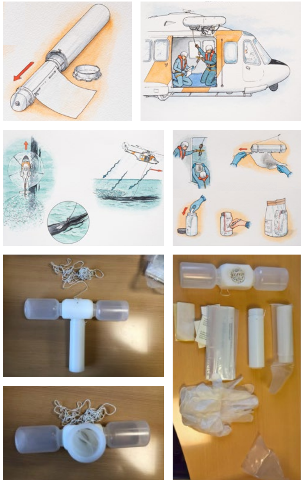
Figure 10: Sampling device set for oil sampling from heights, using a floating device, nylon cylinder and ETFE net. The long white cylinder that is attached to the flotation device has ETFE net attached on the inside with a Nylon strip. Top left image shows the set ready for sampling. Bottom left picture shows the ETFE net inside the nylon cylinder. The Nylon cylinder with the ETFE net is removed from the floatation device after sampling, and packed for analysis. Credits: Danish Defence.
