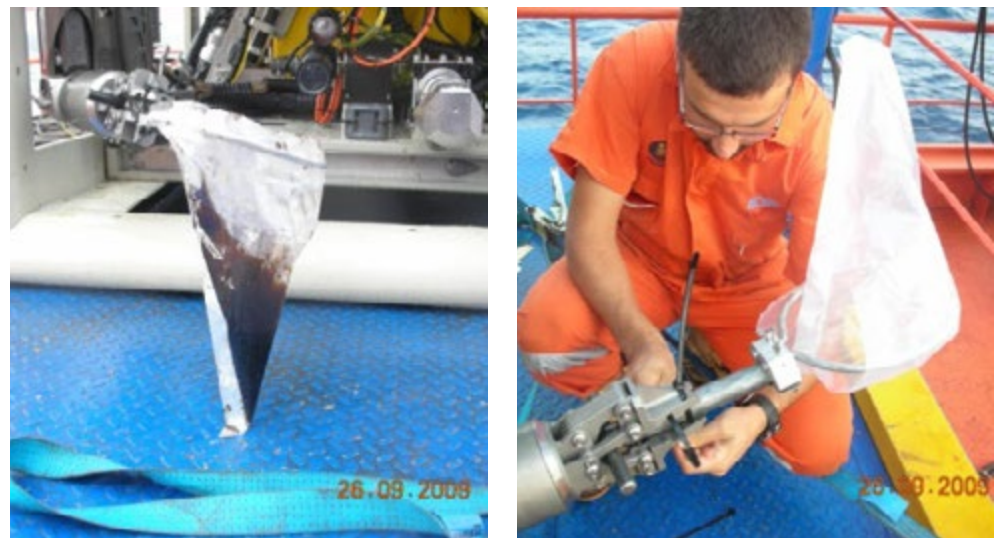
Figure 17: Oil sampling by help of a ROV (credits: SASEMAR, Spain)
